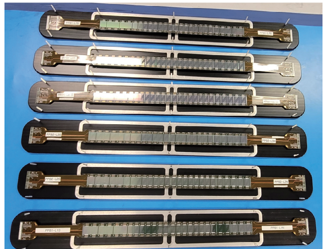
Fig. 2. Fully assembled INTT preproduction ladders.
