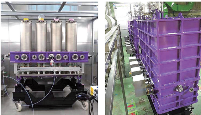
Fig. 7. Photographs of cryomodule. (Left) After assembling and sealing the cavities and beam pipes in the clean room. (Right) After alignment at the installation site.
