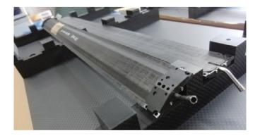
Fig. 1. The CFRP staves for INTT ladder.
