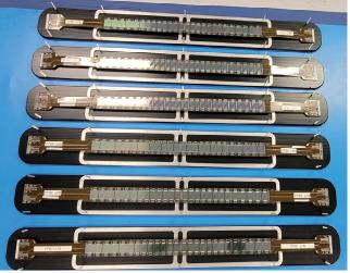
Fig. 2. Fully assembled INTT preproduction ladders.
