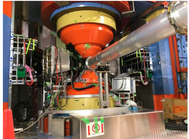
Fig. 2. Photograph of the E16 Spectrometer, which is under construction.
