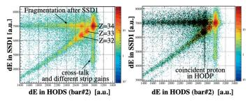
Fig. 2. Charge identification of outgoing fragments in the first SSD and in HODS.
