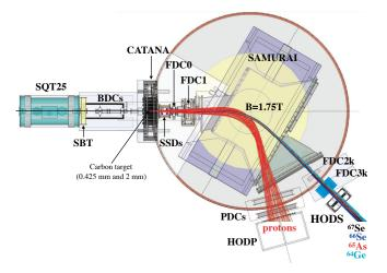
Fig. 1. The experimental setup in NP1406-SAMURAI24.
