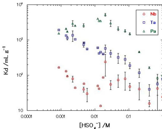
Fig. 1. Variation of the  $K_d$  values of <sup>95</sup>Nb, <sup>179</sup>Ta and <sup>233</sup>Pa on the anion-exchanger CA08Y as a function of HSO<sub>4</sub><sup>-</sup> concentration [HSO<sub>4</sub><sup>-</sup>].
