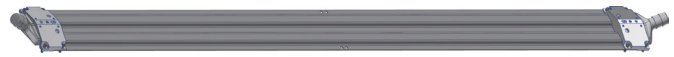
Fig. 3. The auto-CAD drawing of the stave support structure with the air cooling tubes.
