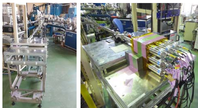
Fig. 2. BL-W15 started to be used again as a multipurpose beam line after the renewal of the beam diagnostic system. The degree of vacuum level for the user setup is required to be better than 10 -4 Pa. (Left). A setup for calibration of gamma ray detectors using a resonance reaction with a carbon target bombarded by 1 or 2 MeV proton beams (Right).
