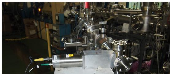
Fig. 2. Experimental setup. Proton beams from the Pelletron accelerator hit a carbon target in the small vacuum chamber, and  $\gamma$  rays were measured by the NaI(Tl) scintillator seen in the center of the photograph.
