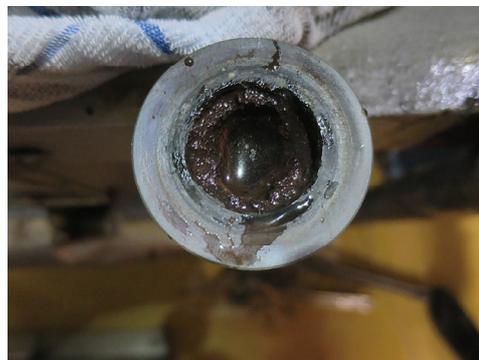
Fig. 1. Blocked cooling water piping for the turbines.
