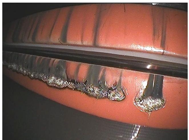
Fig. 3. Damaged correction coil of the DMT3 magnet.
