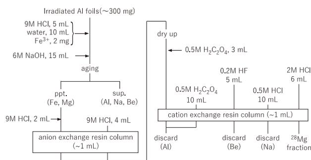
Fig. 2. Chemical procedure for the preparation of no-carrier added  $^{28}\text{Mg}$  tracer.
