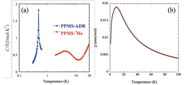
Fig. 1. (a) Temperature dependence of the total specific heat divided by temperature  $C/T$ . (b) Temperature dependence of magnetic susceptibility measured at 1 T (open red circles). The grey solid line represents the theoretical curve of the linear spin chain model with a AFM interaction  $J = 15.5 \text{ K}$ .
