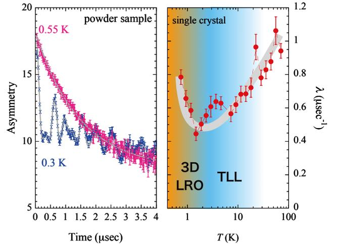
Fig. 2. (a) Selected ZF- $\mu\text{SR}$  signals (asymmetry vs time). The gray lines are the corresponding fits to the data. (b) Temperature dependence of the muon spin relaxation rate in  $\text{Na}_2\text{CuCl}_2\text{SO}_4$  measured in longitudinal field 50 G.
