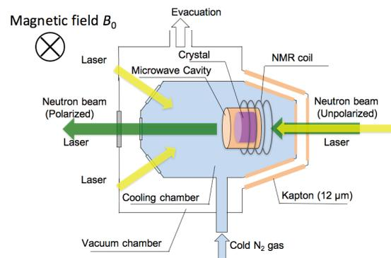
Fig. 1. Setup of the neutron polarization system using Triplet-DNP.
