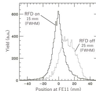
Fig. 3. Beam focusing of  $^{79}\text{Se}$  at FE11 with and without RFD.
