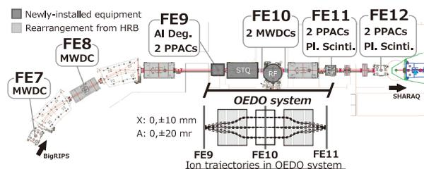
Fig. 1. Schematic view of the OEDO beamline. The ion optics in the OEDO system are also shown.
