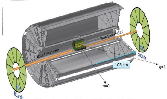
Fig. 1. INTT detector in the sPHENIX tracking system.
