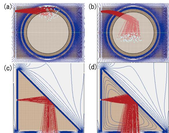
Fig. 3. Simulation results of trajectories of SEs obtained using SIMION 3D. The equipotential lines (blue) and the electronic tracks (red) are calculated with an correction voltage of 0 V (a, c) and  $-350$  V (b, d). MCP is indicated by the white region (a, b).
