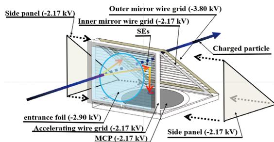
Fig. 1. Schematic view of the TOF detector and typical applied voltage. When the charged particles pass through the TOF detector, secondary electrons (SEs) are emitted from the entrance foil and guided to the MCP along the electrostatic field.
