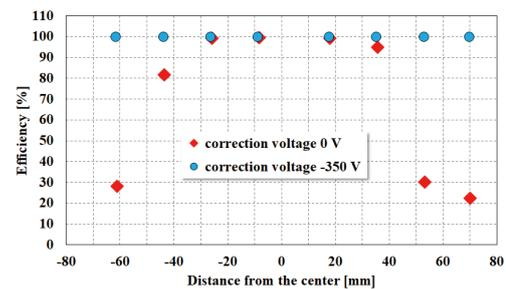
Fig. 2. Measured detection efficiency at the entrance foil in the horizontal space. The horizontal axis indicates the incident position of alpha particles.
