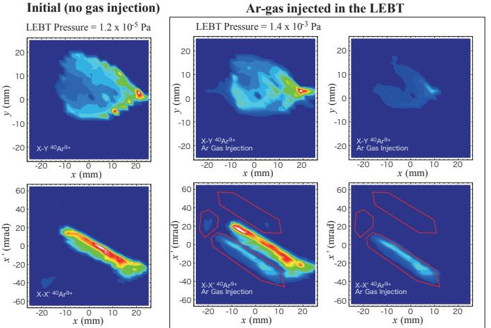
Fig. 2. Obtained beam profile (upper) and horizontal emittance (lower) of  $^{40}\text{Ar}^{9+}$  beam by using PPEM.
