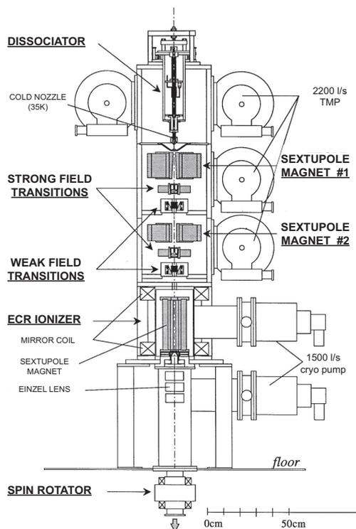
Fig. 2. Atomic-beam-type polarized ion source of RIKEN.
