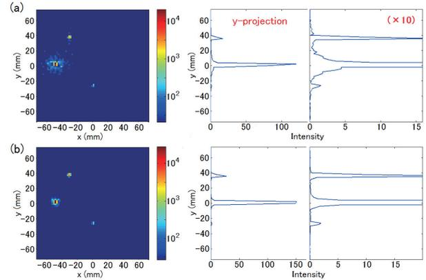
Fig. 2. Reconstructed image of three  $^{22}\text{Na}$  sources with collimators (a) without and (b) with the W-plates. Left is the two-dimensional image, right is its projection to  $y$ -axis and its ten-fold magnification.
