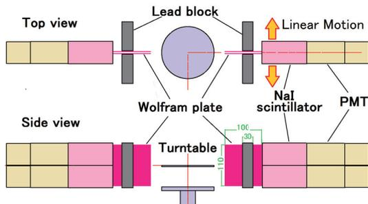
Fig. 1. GIRO detector setup with wolfram plates.
