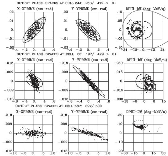
Fig. 1. From top to bottom, results of RFQ, MEBT and IH.
