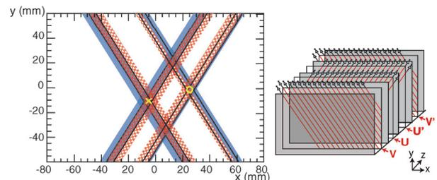
Fig. 1. Example of an event snapshot. The MWDC at F6 consists of 4 planes (U(30°)-U'(30°)-V(60°)-V'(60°)). Solid lines represent hit wires. Blue solid and red meshed bands represent the drift length of U(U') and V(V') planes, respectively. We can track the position (indicated by yellow circle) if there are 4 candidates. The yellow cross denotes the particle in the next bunch of triggered particle.
